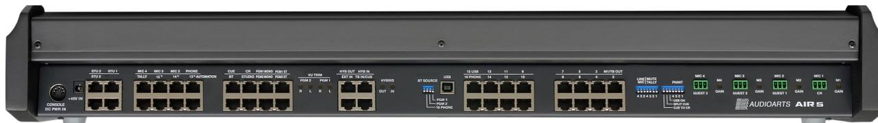
**MIC 1, MIC 2, MIC 3** and **MIC 4** 3-position plug terminals are for mono mic level signals and feed internal adjustable preamps that feed faders 1 – 4.
